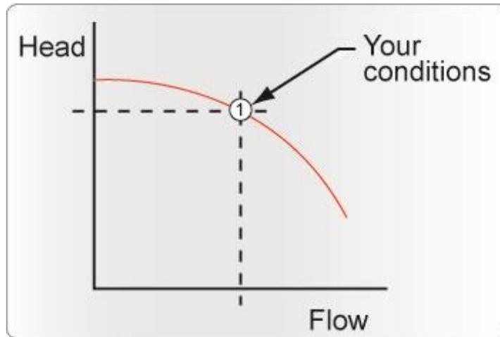
When you find a pump with the flow rate close to your requirement somewhere near the middle of the curve, what leeway do you have with your operating conditions?
