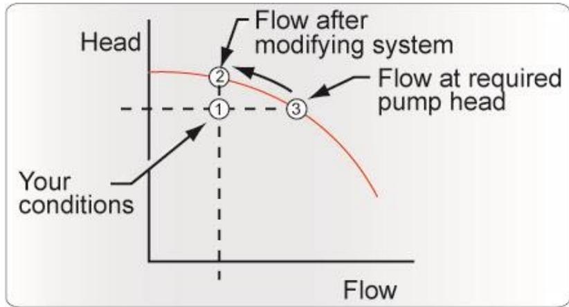
What happens if the pump curve head corresponding to your required flow rate is less than what you need? The pump is not suitable and you need to find a bigger pump or alternatively change something in the system such as increase the pipe size to reduce friction or lower the static head.
