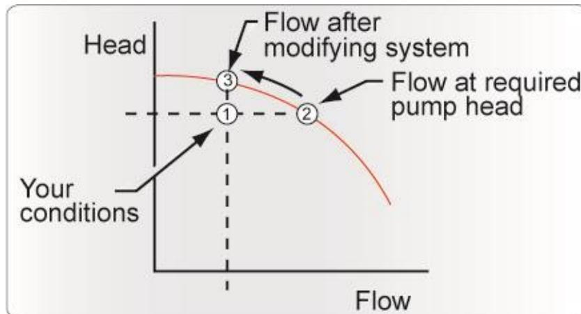
What happens if the pump curve head corresponding to your required flow rate is higher than what you need? You will have to accept more flow (point 3) or change something in the system such as: add a discharge valve and partially close it, reduce the diameter of the pipe sizes or reduce the static head so that you will operate at point 2 on the performance curve.
